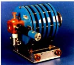
SUPERNANOGAN: An ECR source with permanent magnet for low and high charge state. ( H^+ : 2mA, Ar^{6+} : 350 \mu Ae)
